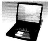
A **laptop** (also called a **notebook PC**) is a lightweight computer that you can transport easily. It can work as fast as a desktop PC, with similar processors, memory capacity, and disk drives, but it is portable and has a smaller screen. Modern notebooks have a **TFT** (Thin Film Transistor) screen that produces very sharp images.
