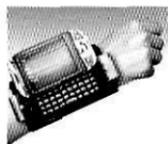
A **wearable computer** runs on batteries and is worn on the user's body, e.g. on a belt, backpack or vest; it is designed for mobile or hands-free operation. Some devices are equipped with a wireless modem, a small keyboard and a screen; others are voice-activated and can access email or voice mail.
